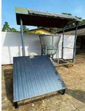
Storage structure with air solar air blower - Solar air heater
