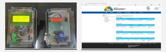
Modified prototype of the sensor-based system (Cluster node in left and sensor node in right)
