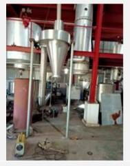
Pneumatic aspiration system for conveyance of granular jaggery
