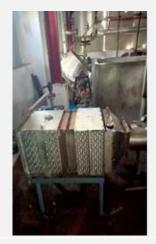
Dehumidifier for removal of moisture from granular jaggery
