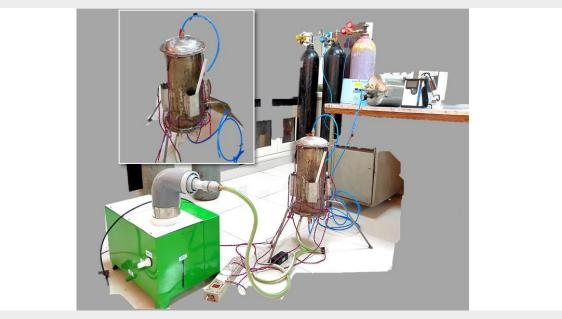
Photoreactor for Ethylene Degradation
