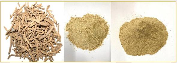
Cryogenically and ambiently ground powder of Safed Musli roots (a: cryogenic b: ambient)
