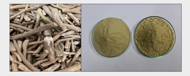
Cryogenically and ambiently ground powder of Ashwagandha (a: cryogenic b: ambient)
