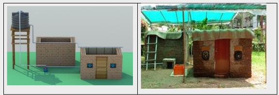
Modified evaporative-cooled chamber
