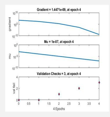
Model validation through gradient and validation checks plots.
