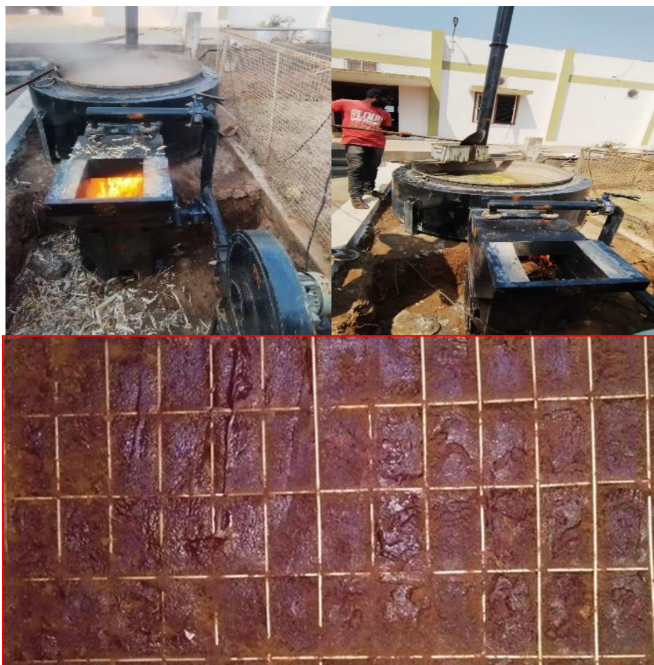
Preparation of jaggery through biomass gasifier
