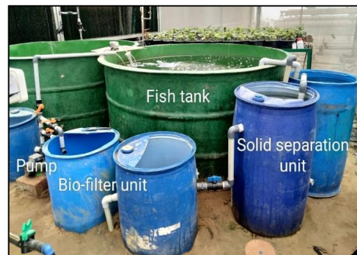
Components of Aquaponics system
