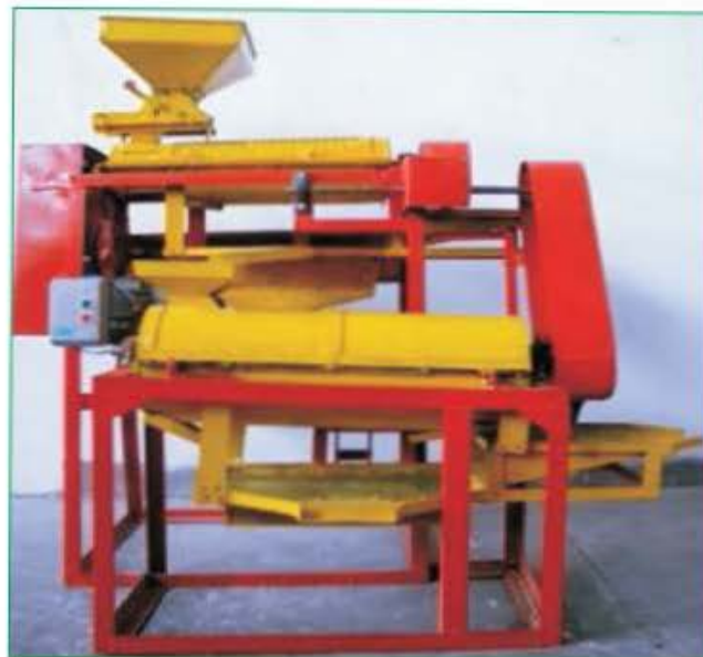
Fig 36. Power operated Scale up maize degermer integrated with pearling system
