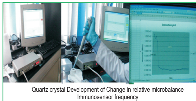
Fig. 4. Detection of pathogen by using QCM based biosensor
