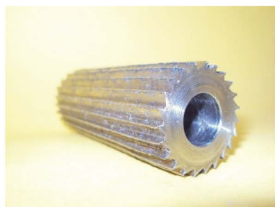
26 slots descaling head (slot depth 2.5 mm)
