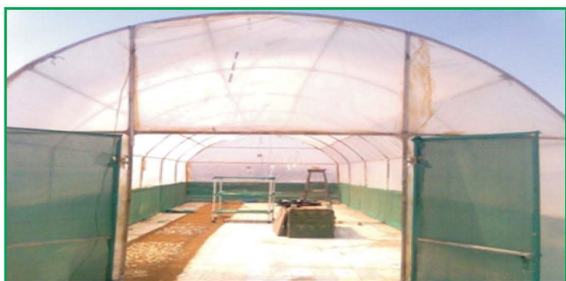
Polyhouse type Tunnel Dryer for fish drying
