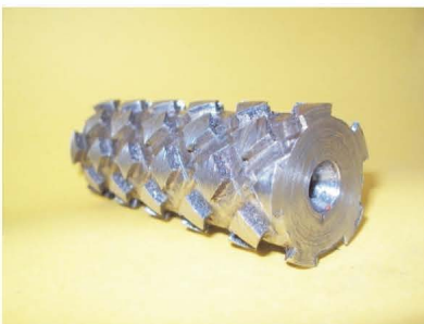
Diamond shaped descaling head (slot depth 2.5mm)
