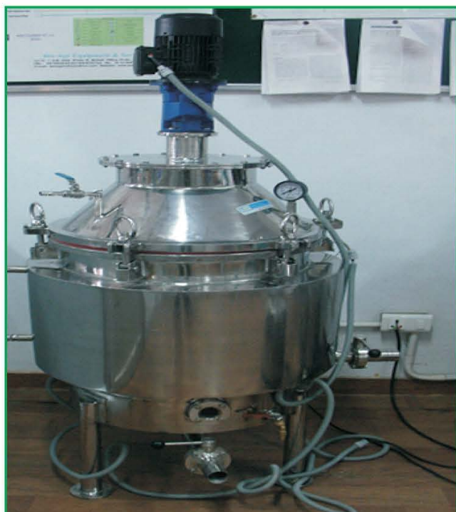
Fig 25: Integrated pilot plant for pretreatment, hydrolysis and fermentation for production of value-added products from crop residues
