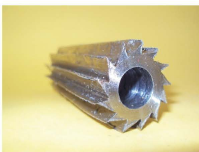
13 slots descaling head (slot depth 5 mm)
