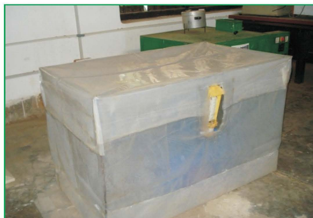
Plastics mango ripening chamber
