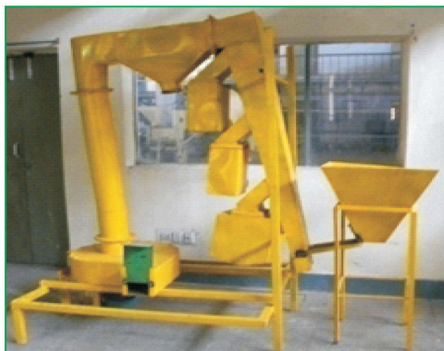
Fig.37a: Aspirator grader (berseem-chicory seed separator), prior to modifications
