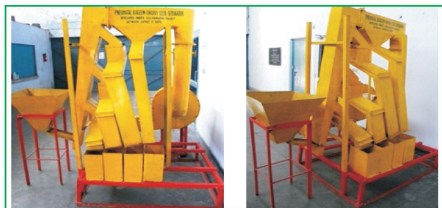
Fig.37b: Berseem-chicory seed separator after modifications
