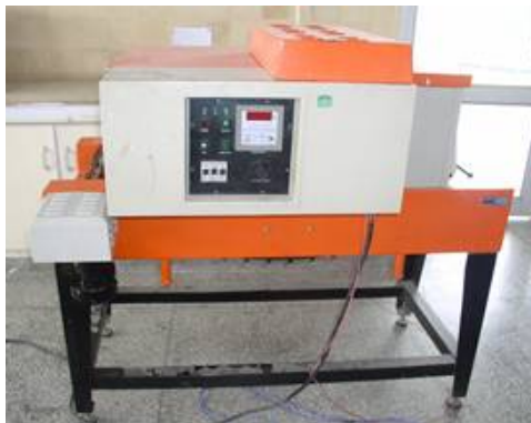
Shrink Wrapping Machine: Wrapping of fruits and vegetables and other products using different plastic films
