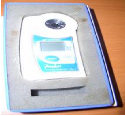
Refracto-meter: To measure total soluble solids (Brix)
