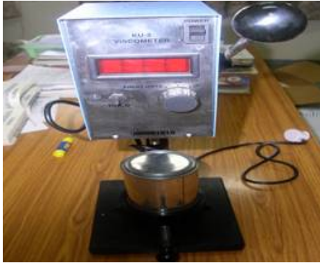
Viscometer: Determination of viscosity of samples
