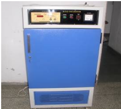
Incubator: For growth of microorganisms at particular temperature
