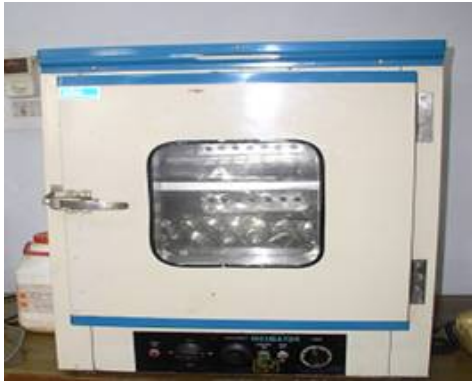
Universal Oven: To measure moisture content of samples and sterilization of glass- wares
