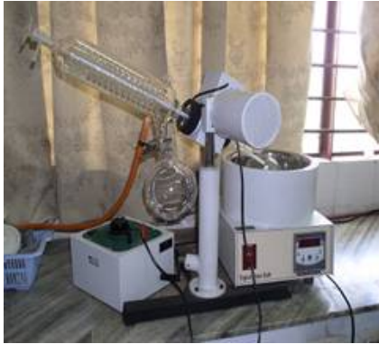
Vacuum flask evaporator: To do evaporation under vacuum
