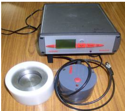
Water activity meter: to measure the available water in food
