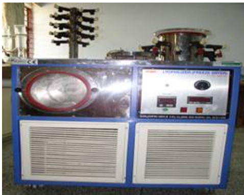
Lyophilizer: For drying of samples at ultralow temperatures
