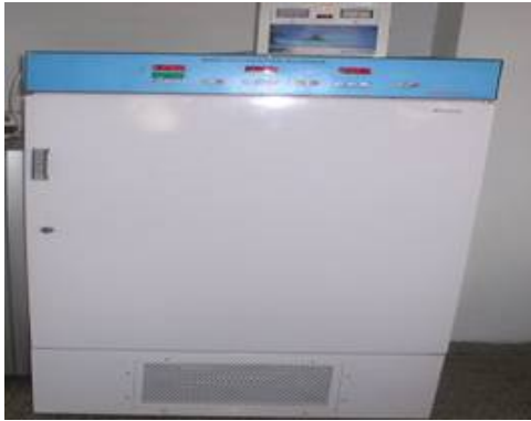
Incubator cum shaker: For growth of microorganisms at particular temperature under shaking condition
