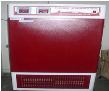
Deep freezer: For preservation of samples and costly chemicals at ultralow temperature
