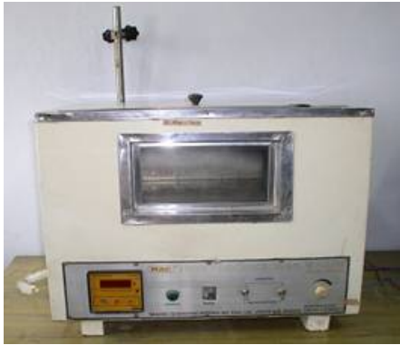
Water bath: During analytical experiments to give a particular temperature
