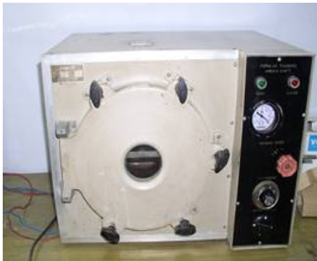
Vacuum dryer: Drying of food samples by vacuum
