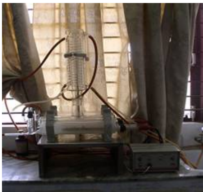
Distillation assembly: For preparation of distilled water
