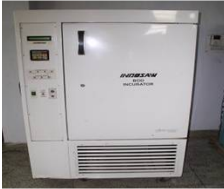
BOD Incubator: Incubation could be given for the growth of specific microbes with specific heat and relative humidity.
