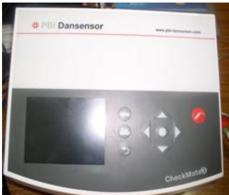
Headspace gas analyzer –Estimation of gas concentrations in MAP food
