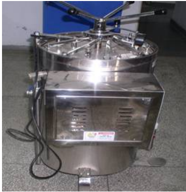
Autoclave: Sterilization of glasswares, media etc. for microbiology purpose
