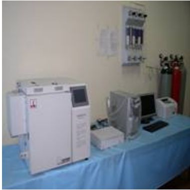
Gas Liquid Chromatography: Separation and quantification of volatile components and pigments
