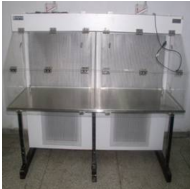
Laminar air flow: For aseptic maintenance and transfer of microorganisms cultures
