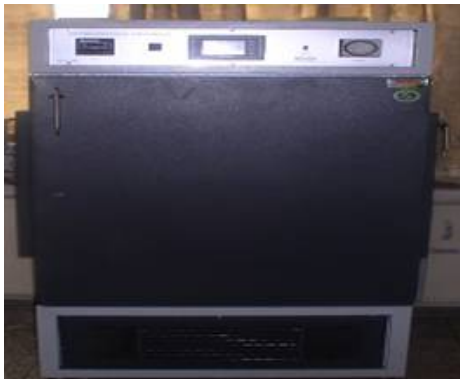
Environmental Chamber: For growth of microorganisms at different environmental conditions
