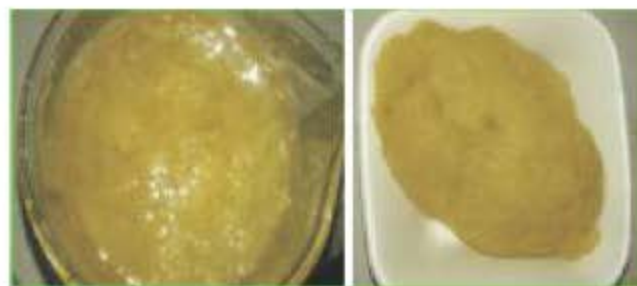
Fig. 62: Figure showing precipitation of pectin from citrus crude extract
