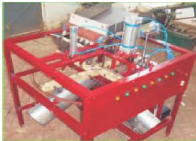
Fig. 70. Prototype view of ber decoring machine
