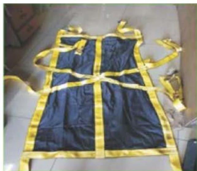
Fig. 7. Modified design of animal lifter
