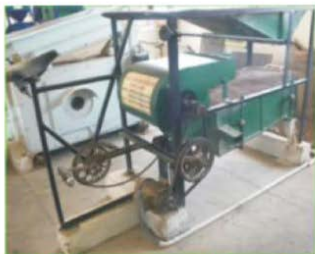
Fig. 26. Pedal cum power operated air screen grain cleaner cum grader
