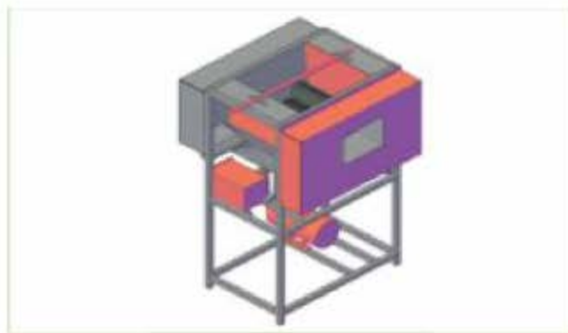
Fig. 33. Taro peeling machine design
