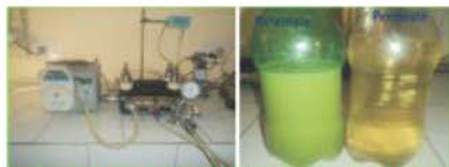
Fig. 61: Process of ultrafiltration, permeate and retentate
