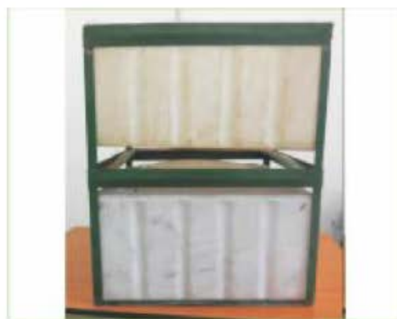
Fig. 74. Stackable live fish transport container
