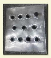
Fig 2. PCM chamber for thermal storage
