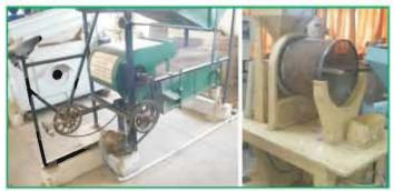
Fig. 8: Pedal cum power operated air screen grain cleaner cum grader
