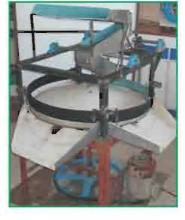
0.3% damage. Capacity of the machine at 25 RPM was 400 kg/h for aonla. It is operated by 1 hp electric motor. The machine costs about Rs. 50,000. This fruit grader is suitable for both at farm level as well as commercial level operations.
