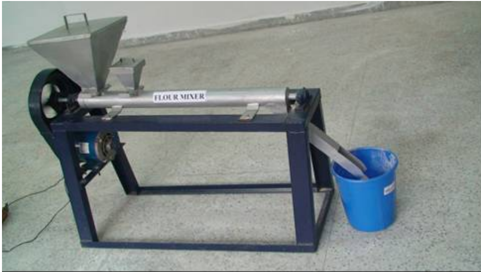
Low cost flour mixer developed at CIPHET for production of composite flours and micro nutrient enriched flours
