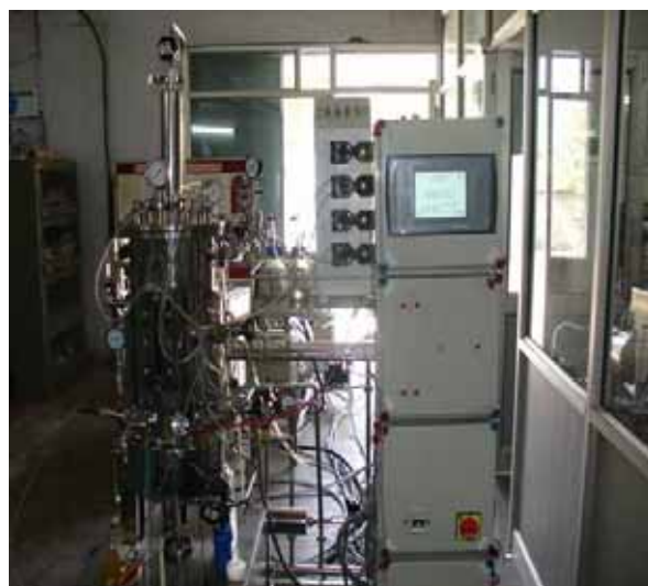
Fermenter of 30 litre capacity with controls for temperature, pH, DO and CO 2 monitoring installed at CIPHET, Ludhiana
