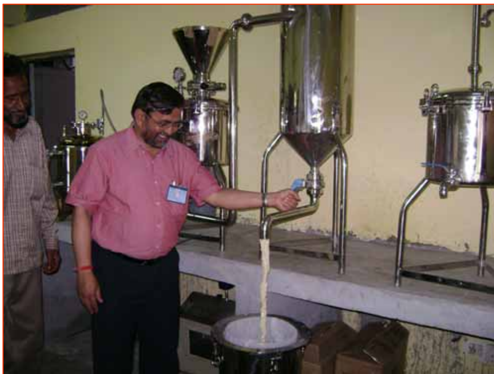
The modern processing plant with airless grinding and deodorizer to get flavour free ground nut milk at CIPHET Ludhiana
