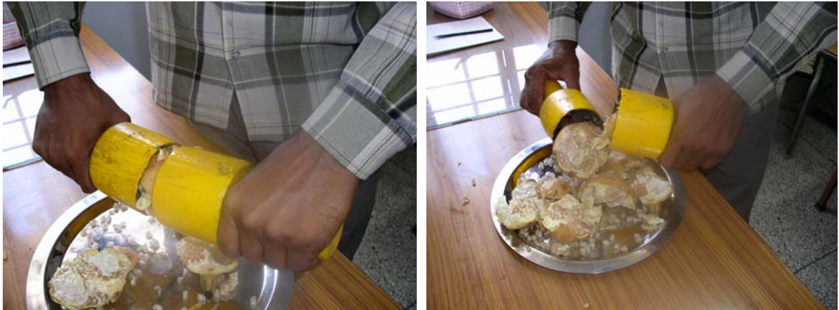
Figures: Working with hand tool for easy separation of arils from pomegranate
