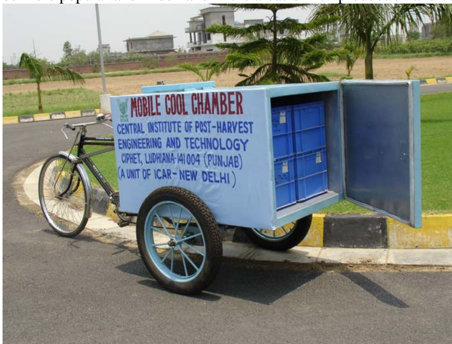
Mobile cool chamber on cycle rickshaw for fish storage, transportation, and retail marketing
